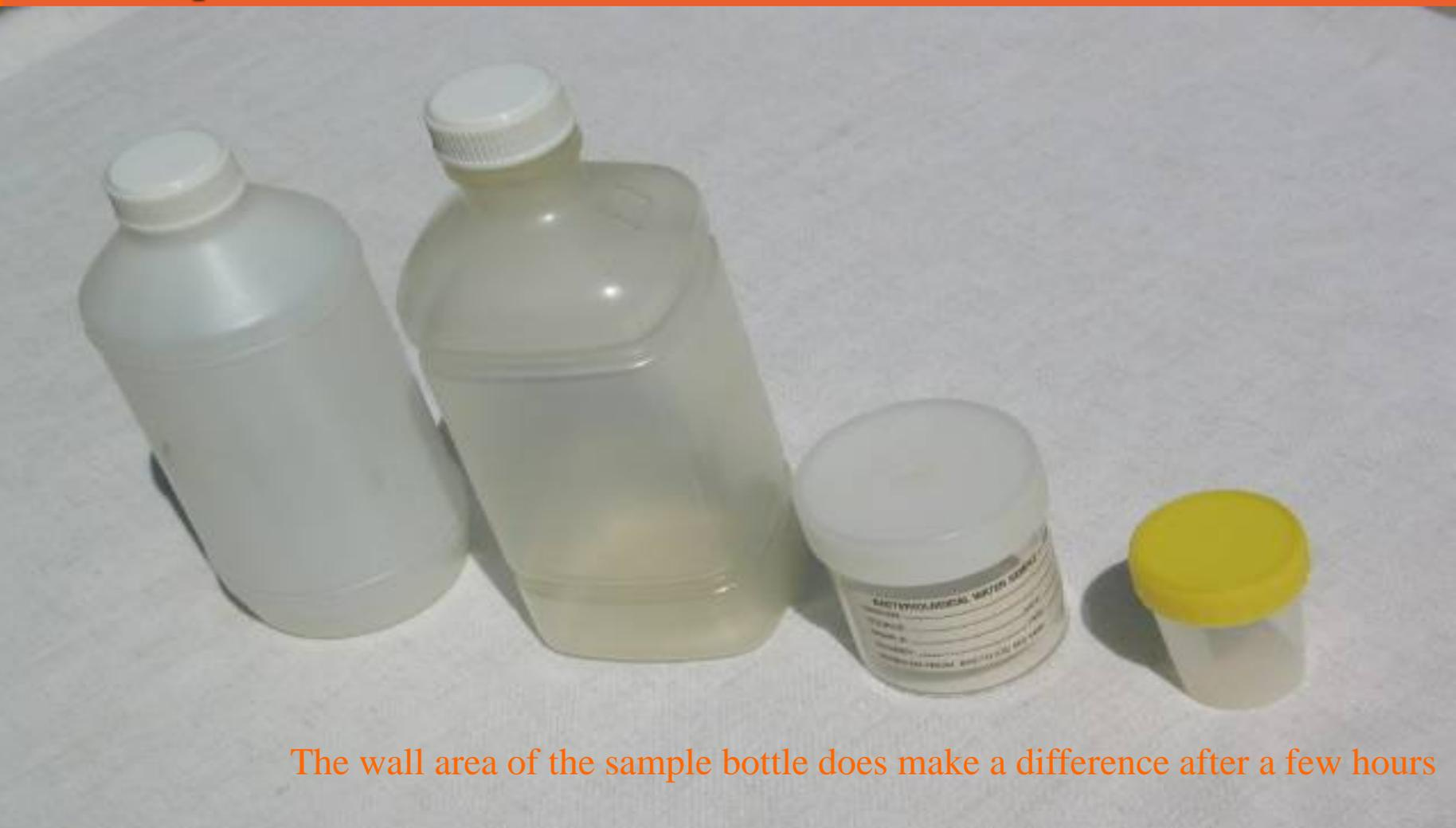
The wall area of the sample bottle does make a difference after a few hours
