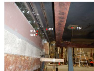
Figure A4.3: Bottom side: Unexposed side (red) thermocouple locations
