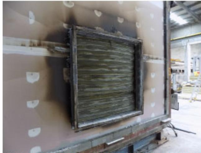
Figure A6.4: Unexposed face of specimen after removal of the connecting duct, post-test.
