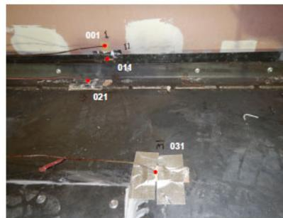
Figure A4.5: Top side: Unexposed side (red) thermocouple locations
