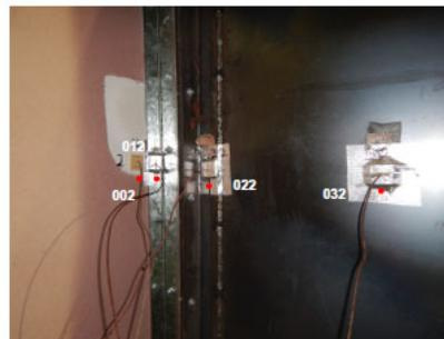
Figure A4.2: South side: Unexposed side (red) thermocouple locations
