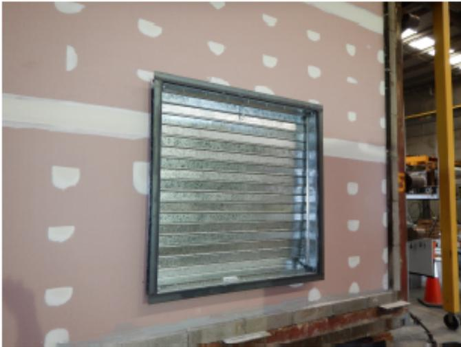
Figure A6.1: Unexposed face of specimen at completion of the pre-exposure cycling.
