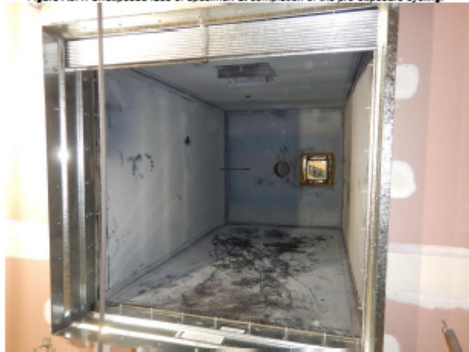
Figure A6.2: Exposed face of specimen before the heating period.
