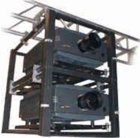
**Dual convergence** is the method of superimposing the images from many projectors to make a single composite image. Specially designed projector mounts allow projectors to be stacked and properly positioned. Adjust the image using the lens shift function, the mount's pan, and tilt adjustments. Each image should be projected pixel per pixel over the original image to produce a clear image. This is done to increase the brightness of the projector and it creates a redundant backup projector.
