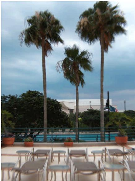
In the image above you can see that the center of the image is in focus while the sides and corners are fuzzy. A damaged or improperly installed lens may cause the corners of the image to appear fuzzy.
