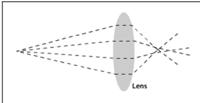
If the projector's image appears to be out of focus in some areas but in focus in others, and you are using the lens shift function, your image may be poor due to spherical aberration. To improve the image put the lens back in the neutral position so that it's lined up with the optics. Move the projector so that it's square to the screen and see if the image improves.
