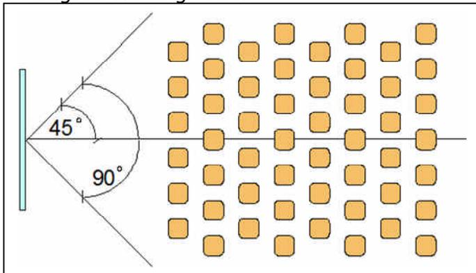
In many events, the width and/or depth of the audience will exceed the ideal viewing area of the image. One obvious solution is to get a larger screen, but often factors such as ceiling height prevent you from increasing the image size. In these situations, placing repeater screens along the parameters of the event space will help the entire audience view the image.
