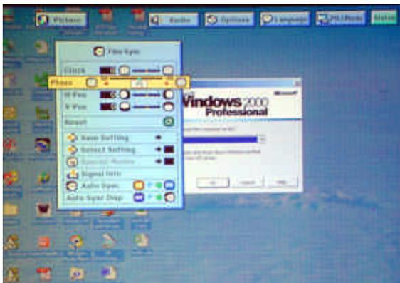
This is a photograph of an image that needs the phase control adjusted. Note the horizontal lines in the background of the image.
