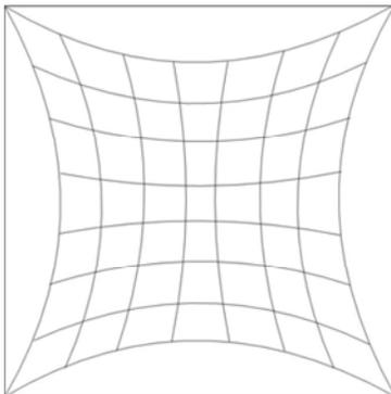
Lens shift may cause a pin cushioning effect, which the image appears to be concave around the edges. Of course, pin cushioning doesn't always appear equal on all sides of the image. If it is combined with a keystone effect, the image may be pin cushioned on only one side. The best solution these optical effects is to properly orient the projector to the screen.
